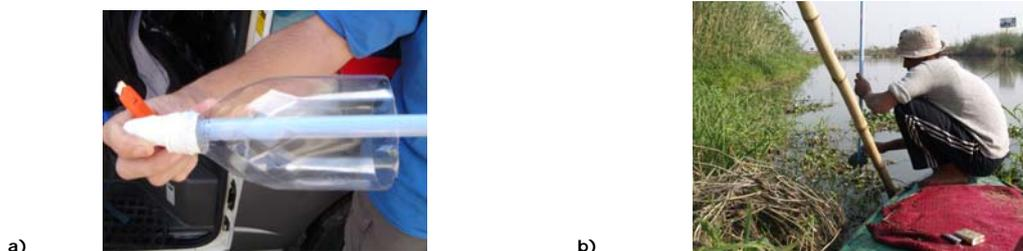
**Figure 5.** Sediment sampling methods used. a) Plastic small container to sample the sediment from the bottom of the lake Mariut. b) Sediment sampling in the lake Mariut.
