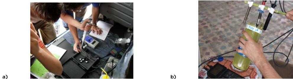
**Figure 2.** Water analysis. a) Nutrients and heavy metals evaluation by means of a field photometer. b) Physical water conditions evaluation by the use of three different sensors (oxymeter, pHmeter and conductimeter).
